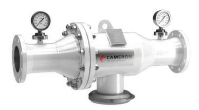
The rock catcher is a safeguard in the bulk transfer system, reducing the wear and tear on the system as well as preserving the uniformity of the bulk powder. The rock catcher prevents oversized objects from entering the onboard bulk system during bulk transfers from supply vessels. It also breaks any large lumps of bulk material into finer, more manageable pieces.
