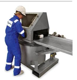
The CMU is designed as a fully transportable unit with integrated forklift supports and manual operation to provide quick and hassle-free relocation whenever required.
