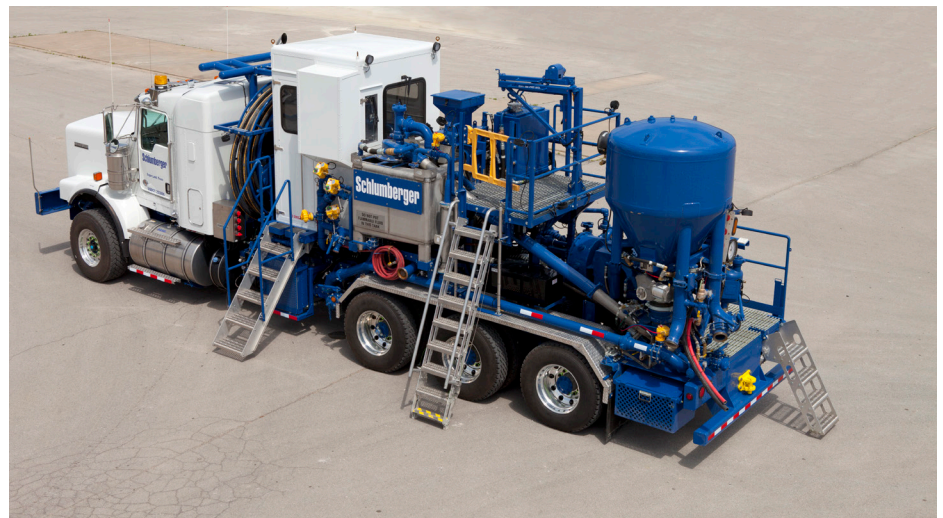
CPT-179 single-pump cement truck.†
