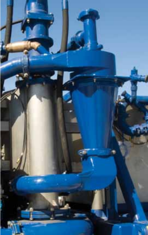
The SlurryAirSeparator tool requires no power supply and has no moving parts, making it easy to install and maintain.
