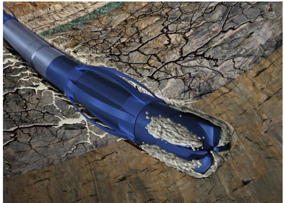
ThixoCRETE solution stops circulation losses in fractured and vuggy formations by rapidly developing gel strength and compressive strength.
