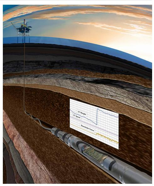
Tension and compression measurements in real time ensure shifting tools are properly engaged, and provide confirmation of shifting sleeve activation.
