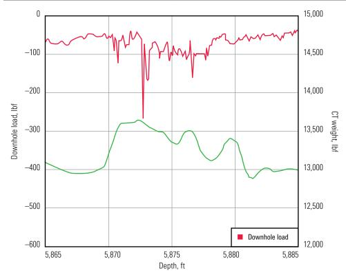
Spike in downhole load curve provides confirmation of shifting of sliding sleeve; no indication is seen on the CT weight measurement at surface.
