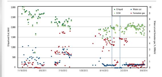
Schlumberger recommended bullheading a 12.5% concentration of B-355 asphaltene inhibition treatment; post-treatment well production was restarted using coiled tubing nitrogen lift.
