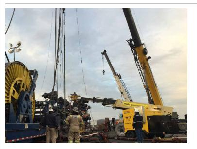
To minimize costs and mitigate risk, Schlumberger recommended CoilTOOLS tools and solutions to rig up the 24-ft packer assembly using CT instead, eliminating a redundant crew and truck on location. Schlumberger sourced the swivel connection and knuckle joints to make up the packer horizontally, allowing the operator to mill out 21 wells and set packers after milling operations with the same crew. This brought average job time down to 10 hours and saved a total of USD 395.000.
