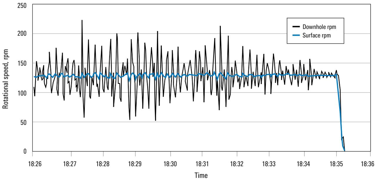
*A postrun visualization of surface and downhole rpm was used to evaluate the effectiveness of a surface control system to minimize stick/slip. The chart was created using high-resolution (50-Hz) data recorded by the OptiDrill service.*
