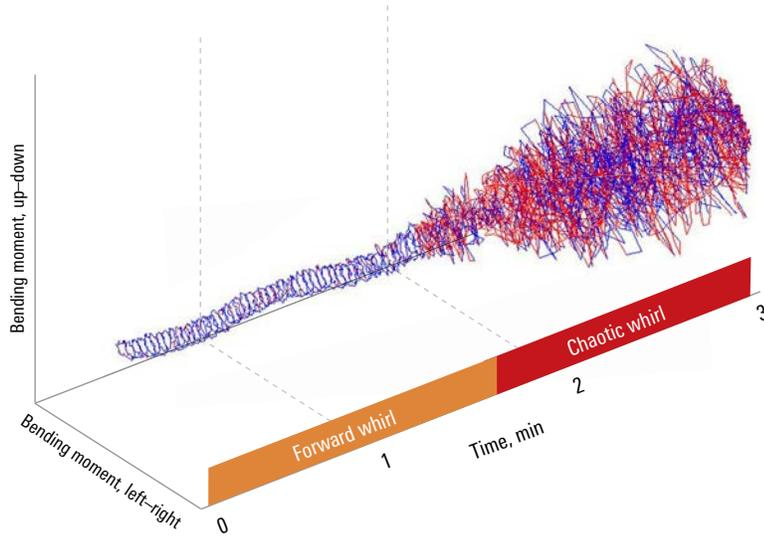
*A BHA with a reamer entered forward whirl motions and then chaotic whirl motions, which were detected and mitigated in real time. Postrun analysis revealed that the whirling motions occurred when the reamer entered an unstable formation. This information will be used while drilling future wells planned in this formation.*
