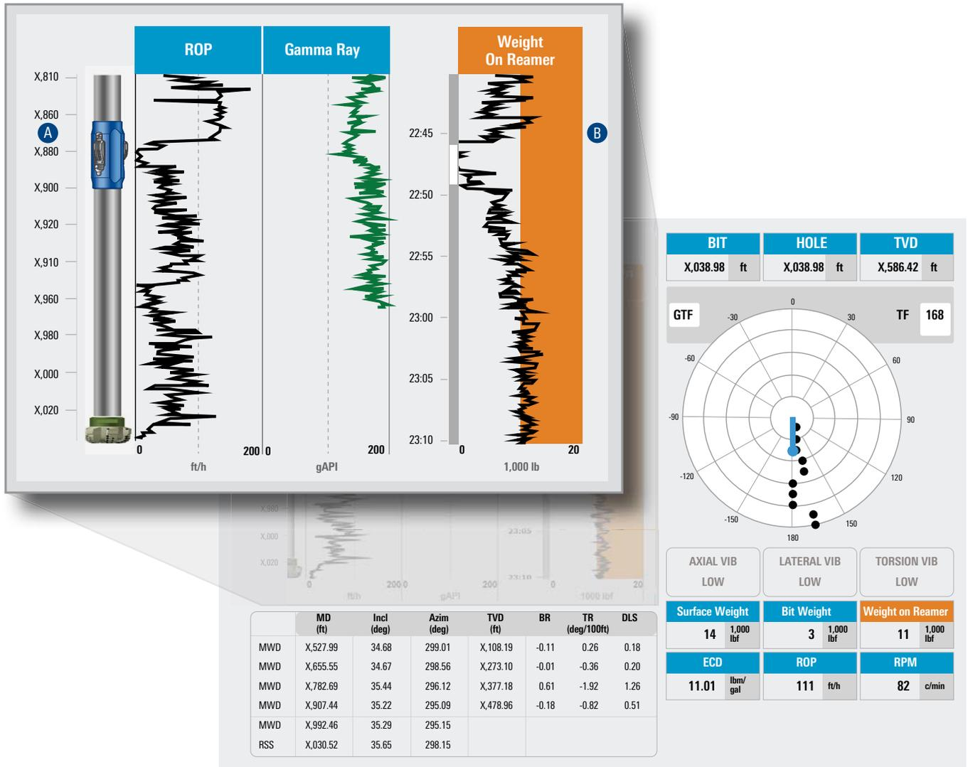
**A** Visualization of the location of the reamer in the formation to help determine cause of change in weight on reamer
