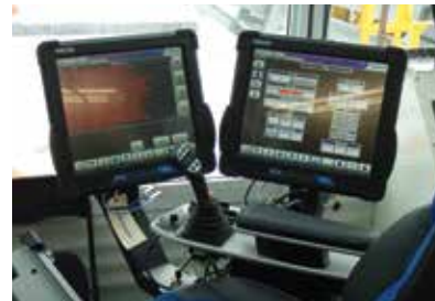
Controls for the implementation of closed-loop drilling automation.
