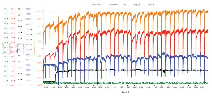
Using the drilling approach recommended by Schlumberger experts, Shell consistently drilled at 180 rpm and applied approximately 60,000-lbf WOB at surface. As a result, Shell achieved a record 275-ft/h average on-bottom ROP and 350- to 390-ft/h [107- to 119-m/h] instantaneous ROP.
