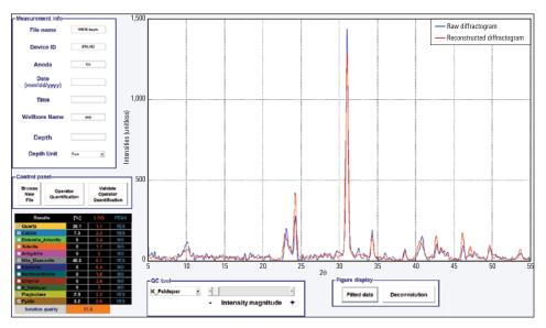
Automatic mineralogical quantification performed by proprietary software shows a close match between the raw and reconstructued diffractograms. This indicates that all minerals have been identified.
