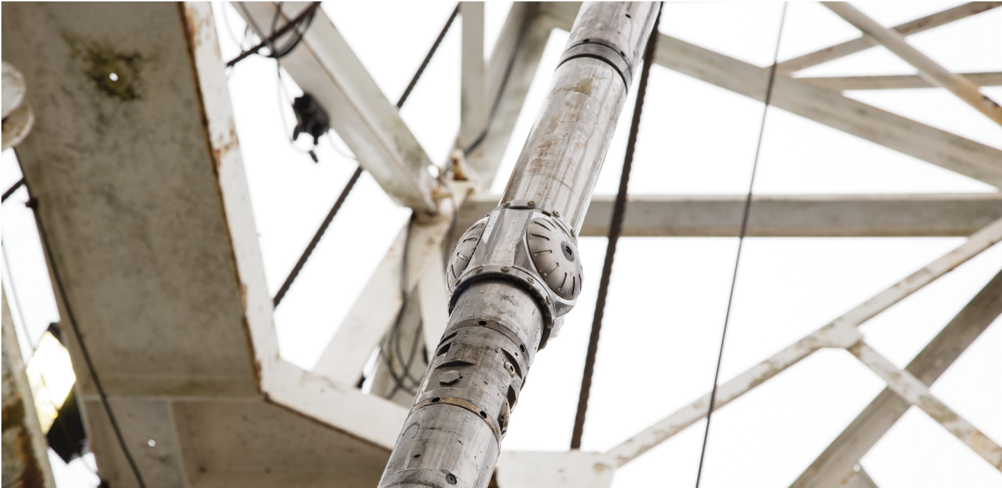
The WellSKATE tri-roller included on an MDT sampling string maintains two of the three wheels in constant contact with the wellbore, which not only reduces the surface contact area to prevent differential sticking but also provides an excellent static friction breaking effect when moving off a station after several hours of sampling.
