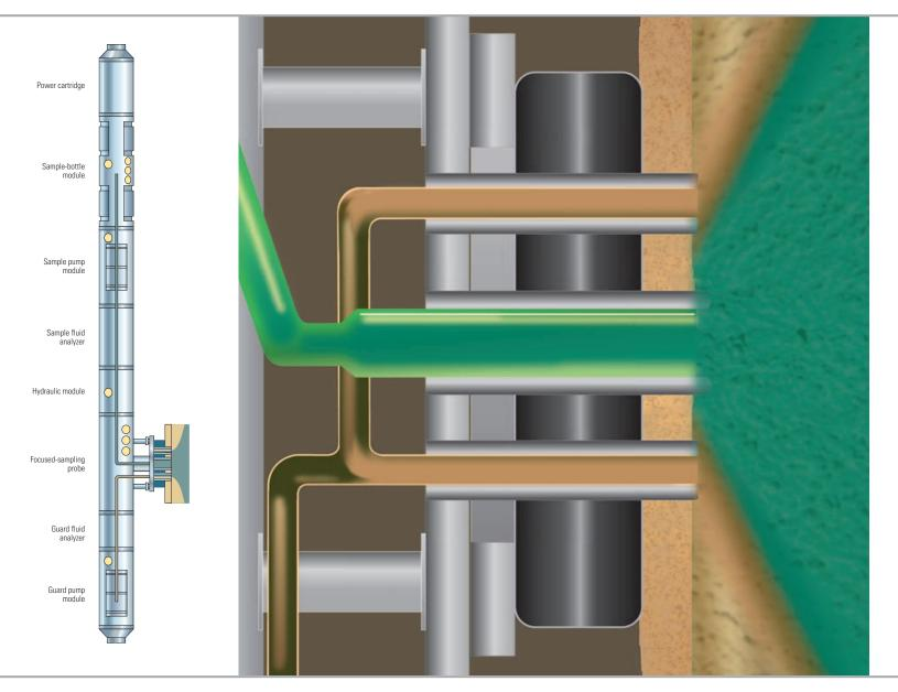
As fluids enter the Quicksilver Probe tool, contaminated fluids flow downward through the guard fluid analyzer and pump while clean fluids flow upward through the extraction fluid analyzer and pump modules to the collection and storage module. Tool configuration, such as the pump location, can be changed for different jobs.
