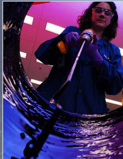
The Saturn 3D radial probe reliably enables sampling of highly viscous oils.
