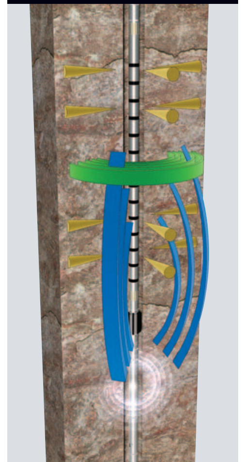
Figure 1. The Sonic Scanner tool provides the benefits of axial, azimuthal, and radial information from both the monopole and the dipole measurements for near-wellbore and far-field slowness information.
