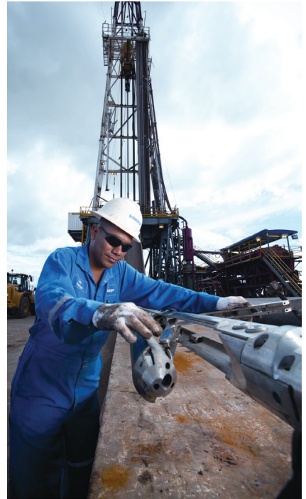
Fig. 2—A Schlumberger engineer inspects the Dielectric Scanner antenna array pad before running the service in a heavy-oil well in South America.
