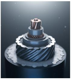
The gas-blocked and torque-balanced StreamLINE iX wireline cable is engineered using the only patented polymer-coating technique, locking the cable core and its armors to form a single element for high integrity in any environment.
