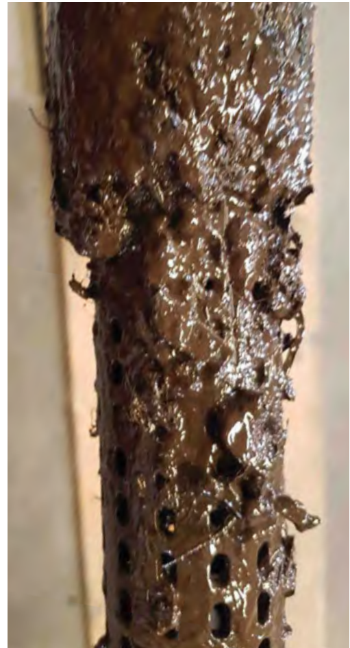
The MUDGARD filter after recovering a variety of potentially damaging debris.
