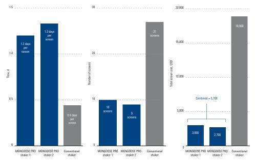
Compared with the conventional shaker, the MONGOOSE PRO shakers enabled longer screen life and used fewer screens over the operation, achieving greater mud recovery efficiency at significantly less cost.
