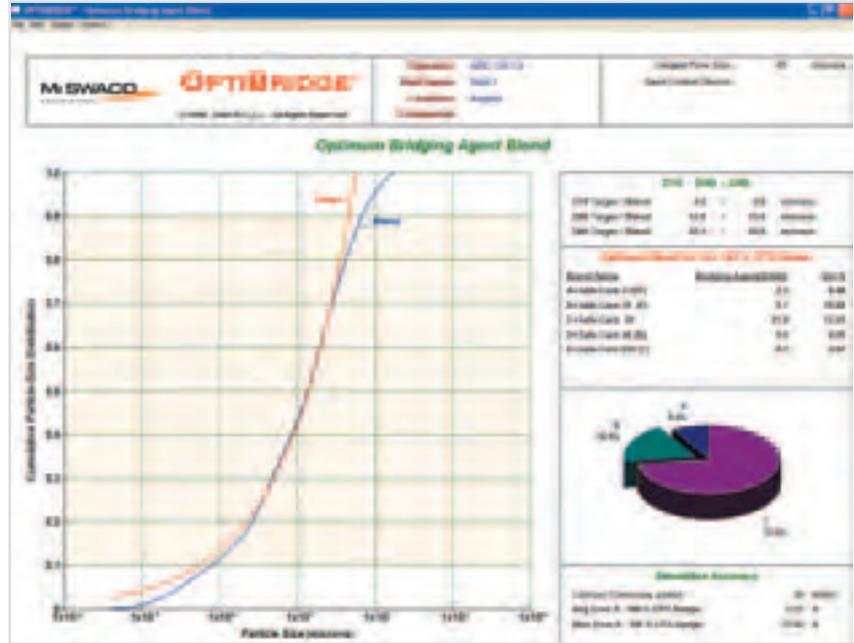
OPTIBRIDGE software generates a target line that defines the ideal blend of locally produced bridging materials that would best fit the targeted formation characteristics. Available anywhere in the world, the OPTIBRIDGE service is an ideal tool for formulating a non-damaging reservoir drill-in fluid. It also can be used to design fracture-sealing and lost-circulation treatments, and to formulate kill and perforation-sealing pills for workover and completion operations.
