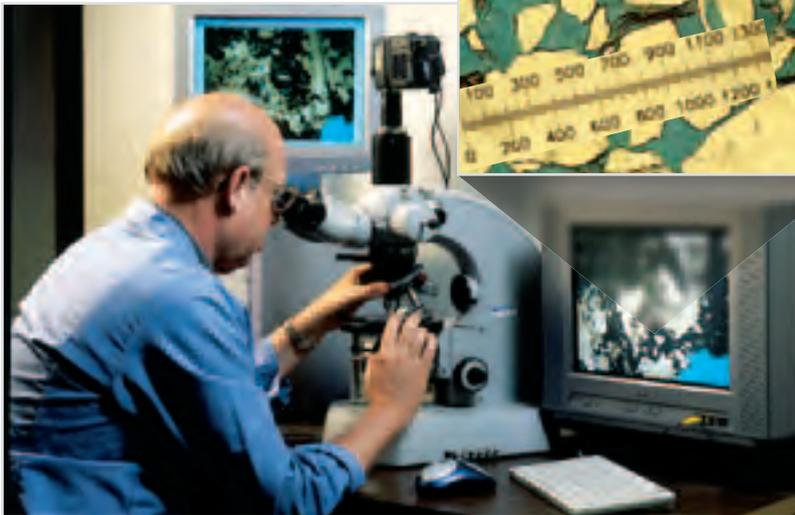
M-I SWACO uses the petrographic microscope to analyze thin sections of reservoir rock materials. Through analysis of pore size and other mineralogical characteristics, we can tailor fluid formulations to specific reservoirs.
