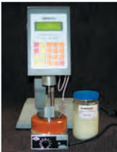
The FLOPRO CT system delivers high LSRVs, which are measured using a Brookfield rheometer. Where extremely high LSRVs are required, a vane spindle is used.
