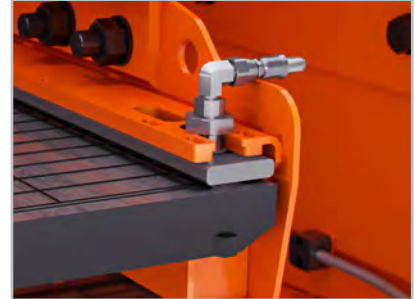
U-shape screen clamping actuators designed with continuous toggle to enable installation from discharge end of shaker
