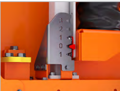
Deck angle can be adjusted while processing fluid. Adjustment range:
