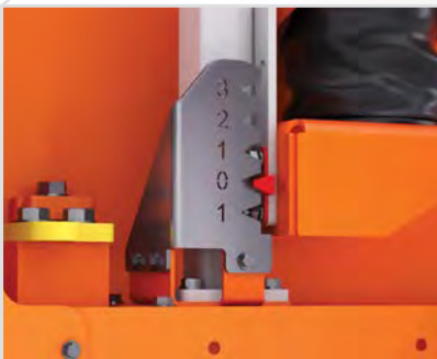
Deck angle can be adjusted while processing fluid. Adjustment Range: - Scalping deck: -1° to +3° - Primary deck: +3° to +7°
