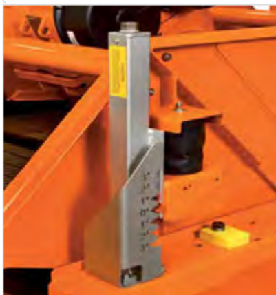
Heavy duty, reliable, mechanical deck adjustment system. Jacks with corrosion resistant coating.
