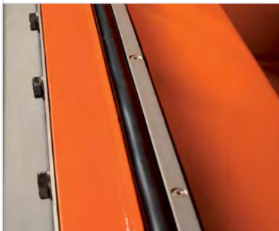
Patented ultra-tight seal between screen and screen bed
