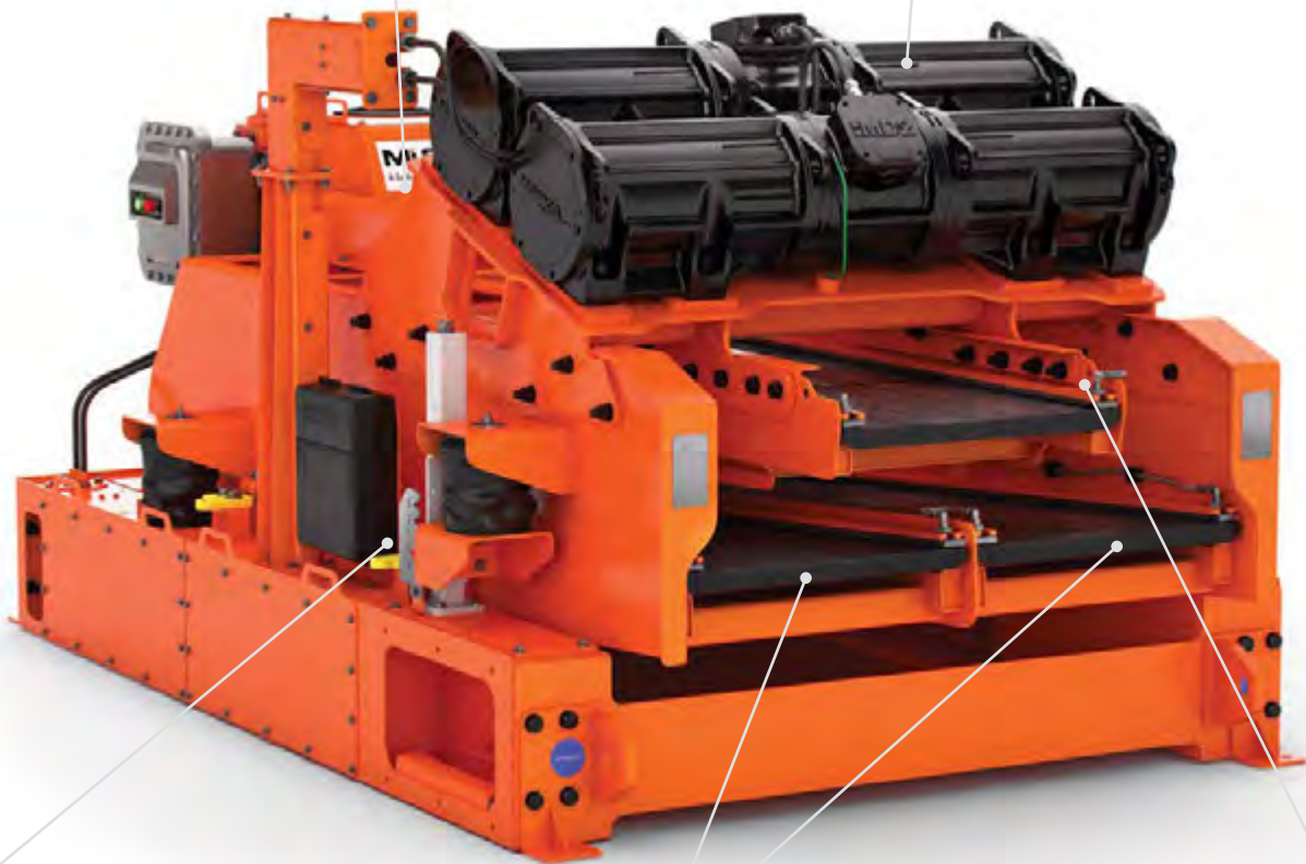
Open access to easily inspect scalping and primary deck screens
