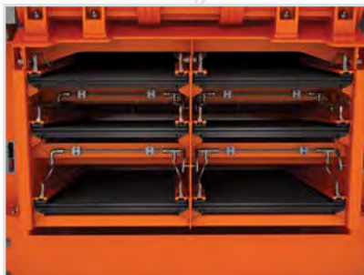
Standard configuration has one scalping deck and two primary decks. Pre-tensioned, composite scalping screens have the following gross screen areas: - Scalping deck: 25.4 ft 2 (2.4 m 2 ) - Primary decks: 50.8 ft 2 (4.7 m 2 )
