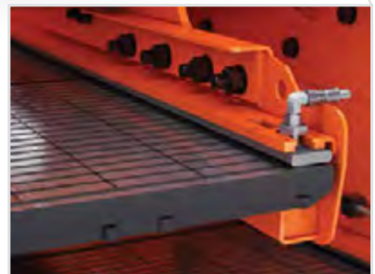
U-shape screen clamping actuators designed with continuous toggle to allow installation from discharge end of shaker
