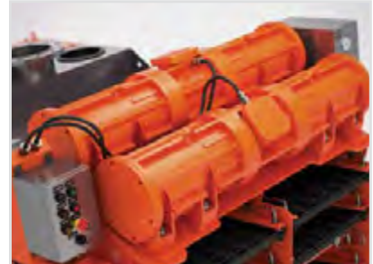
Two state-of-the-art, oilfield proven 3.7-HP motion generators with 1,800 rpm maximum speed
