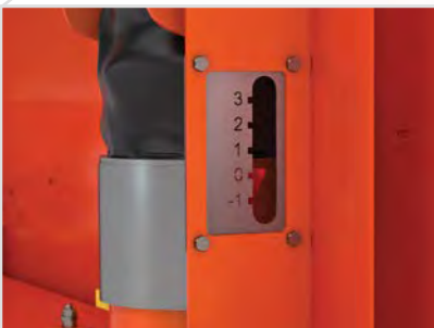
Deck angle can be adjusted while processing fluid. Adjustment range: - Scalping deck: +3° to -1° - Primary decks: +8° to +4°
