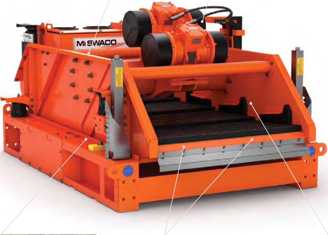
Increased access for inspection, installation, and removal of screens
