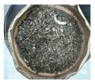
The MAGNOGARD openhole magnet captured more than 30 lb [13.6 kg] of damaging debris during hole enlargement, eliminating the need for a separate cleanup trip. The operator drilled the section to TD in one run, saving 16.5 h of deepwater rig time compared with offset wells where multiple runs were made to achieve the same objective.
