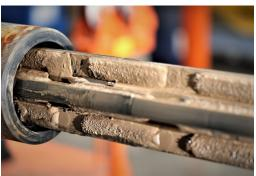
The premium ditch magnets collected 17.6 lb [8 kg] of metallic swarf from the milling operation. The MAGNOSHIELD magnet collected an additional 5.5 lb [2.5 kg] of metallic swarf from the mud system while milling. Also, the MAGNOSHIELD magnet captured a larger piece of debris that could have caused damage to the MWD in the milling BHA.
