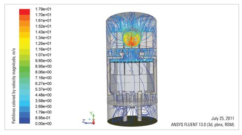
The design of the retrofit scrubber resolved unwanted liquid carryover and increased separation efficiency to maximize design basis throughput.
