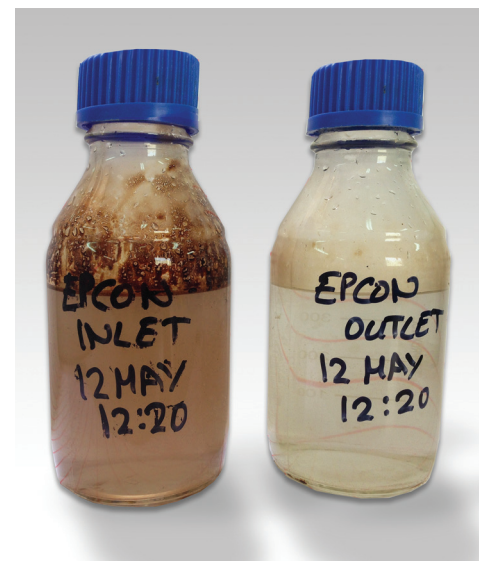
Produced water successfully treated to 10-ppm oil-to-water discharge.
