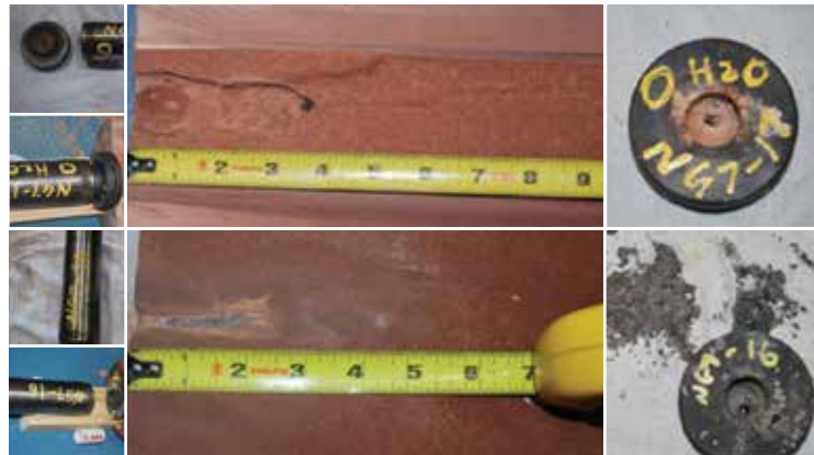
Comparison of split core and casing assembly from 0°-phased test 1 (top) and 180°-phased test 2 (bottom) illustrates the more than 50% improvement achieved in penetration depth.
