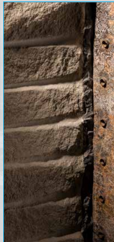
Perforating system performance in a block of sandstone is captured in a polyaxial stress frame.
