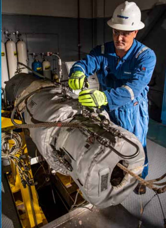
Perforating and flow tests at high-temperature conditions per API RP 19B Section IV quantify dynamic underbalance, depth of perforation, and skin.
