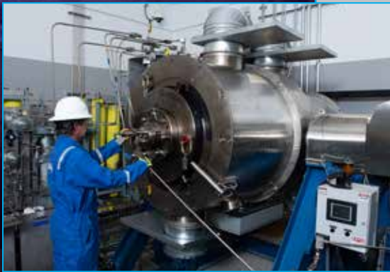
Section IV pressure vessel enables performing testing under extreme high-pressure and high-temperature conditions.
