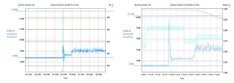
Perforation conducted on conventional high-strength cable (left) experienced 4,400 lbf of shock at the cable-mounted tension device at surface whereas using TuffLINE 18000 cable (right) reduced the peak shock load to 2,300 lbf, significantly lessening operational and safety risk.
