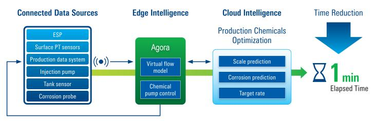
Production Chemicals Optimization on DELFI seamlessly integrates the well's chemical injection system with digital capabilities. Conventional low-frequency manual assessment and adjustment are replaced with real-time monitoring, analysis, and autonomous chemical injection to efficiently manage corrosion and scale.
