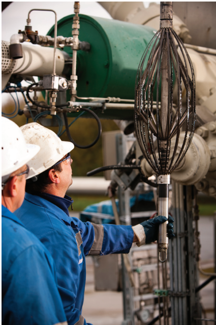
Fig. 1—Engineers examine the 18 pad sensors mounted on the centralizer arms of Schlumberger's EM Pipe Scanner tool before running in a gas well in Europe.
