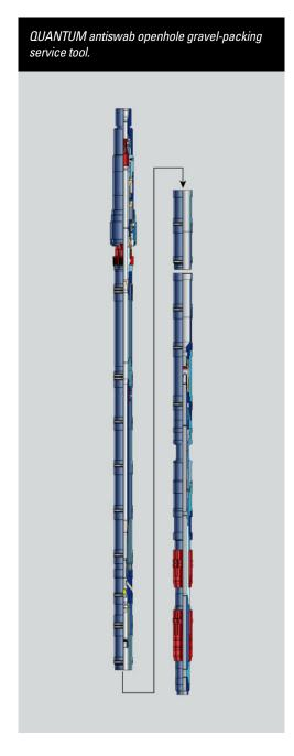
The QUANTUM\* antiswab openhole gravelpacking service tool has been developed to optimize sandface completions in horizontal wellbores by enabling wellbore stability before gravel placement and filtercake cleanup after gravel placement.
