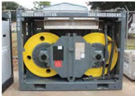
The heavy-duty capstan integrated with the OSU-N unit provides tension relief to increase pull capability.
