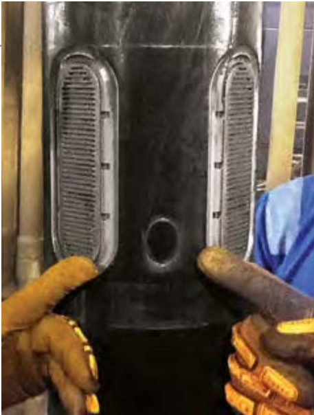
A core imprint of the XL-Rock* large-volume rotary sidewall coring service on a subsequent Saturn 3D radial probe descent in a West Africa well indicates an unsurpassed depth control accuracy of 6 cm with capstan-free conveyance of TuffLINE 18000 cable.
