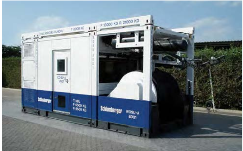
The modular OSU-PA offshore unit is DNV certified capable of pulling up to 18,000 lbf.
