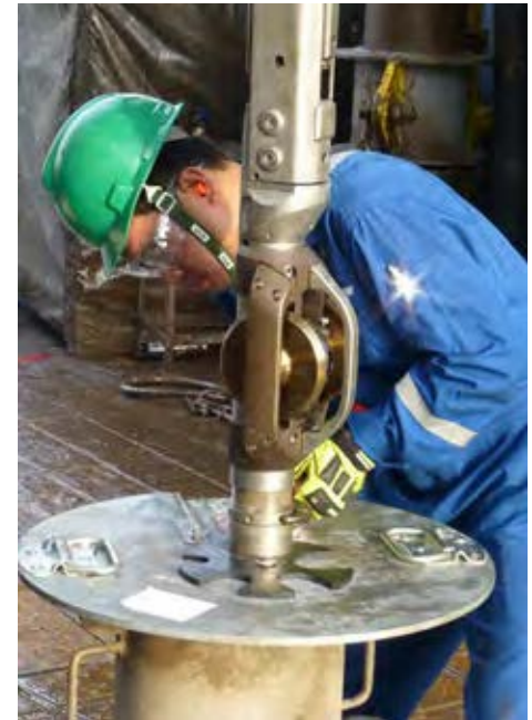
Positively secured to the C spanner recesses of the tool, the Petromac Wireline Express tool taxi provides both low-friction conveyance and orientation.
