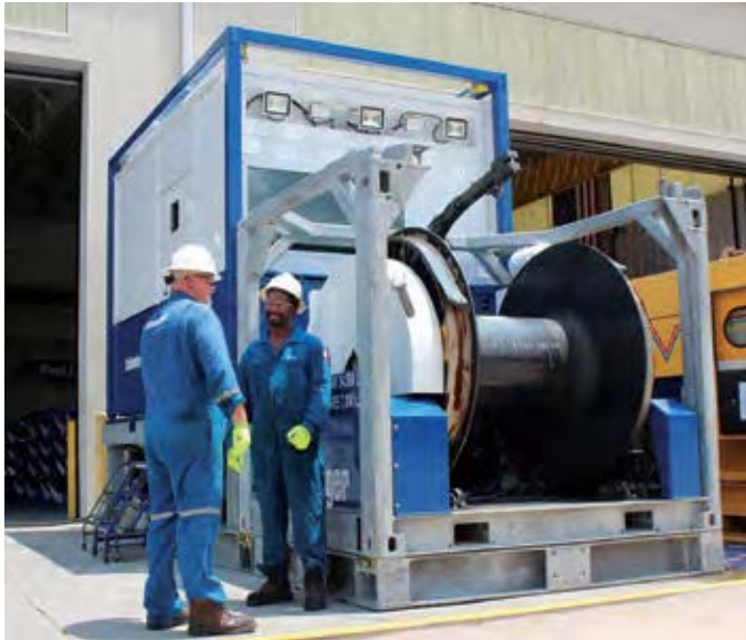
The OSU-N offshore unit deploys TuffLINE 30000 cable from the 43,000-ft capacity WDR-70 drum to increase operational safety and efficiency.
