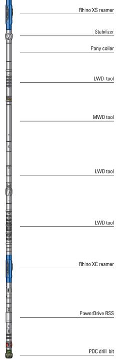
The Rhino RHE dual-reamer system comprises a Rhino XS reamer, a near-bit Rhino XC on-demand reamer, and a PowerDrive RSS paired with a customized PDC bit.
