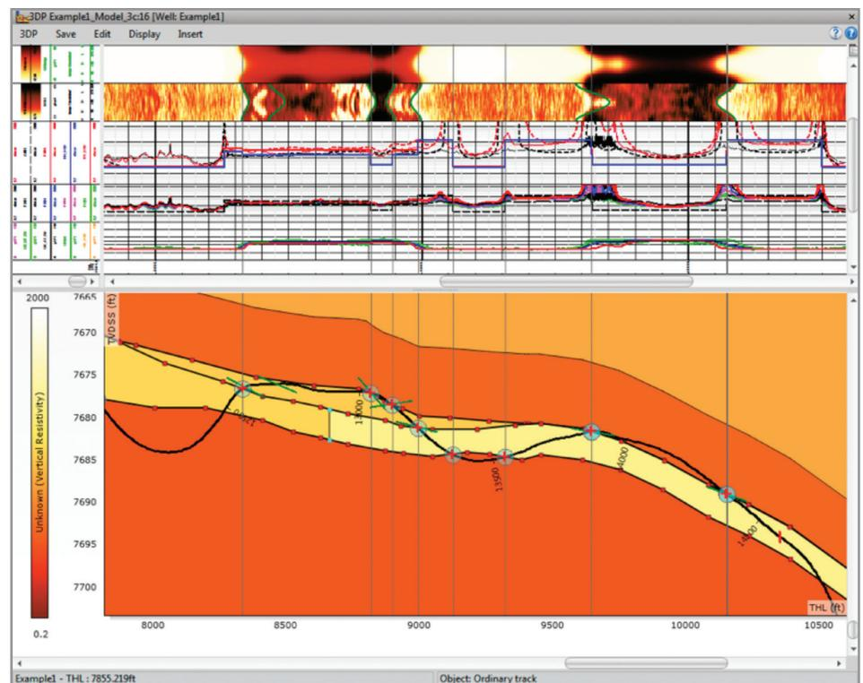
*The measurements acquired in the HAH well are used to define the formation geometry around the well and populate the layer properties.*
