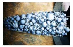
The ultralow-temperature diversion pill improves flexibility and reliability in formations with temperatures as low as 70 degF.
