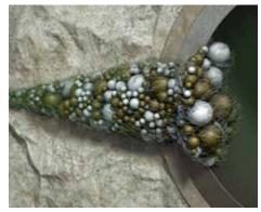
Enhanced-conductivity partially degradable composite pill.
