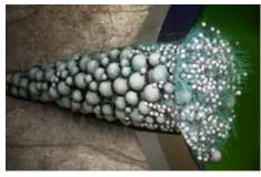
The conventional reservoir diversion pill is designed to promote development of multiple fractures.
