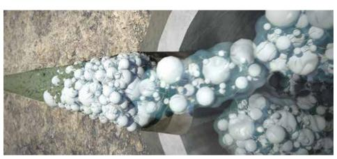
An engineered composite fluid of degradable particles and fibers temporarily isolates fractures at the wellbore.
