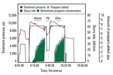
In the interval between two bridge plugs, the BroadBand Sequence service alternates stages of proppant with pills of degradable fibers and particles to improve stimulation effectiveness.
