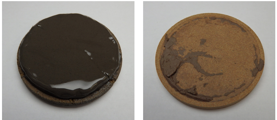
OBM filtercake on a ceramic disc (left) is removed (right) after soaking for 12 h in NaqiClean system at 250 degF [121 degC]. No agitation was necessary.
