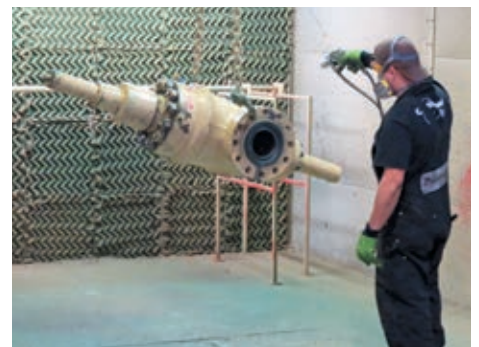
Painted valves are tagged with a test tag verifying repair is complete.
