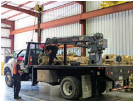
Equipment is offloaded and checked for NORM. The customer and well name are documented and part number and serial number are verified.
