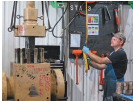
Dedicated cells are set up to follow defined QA for frac valves. The technician begins disassembly.
