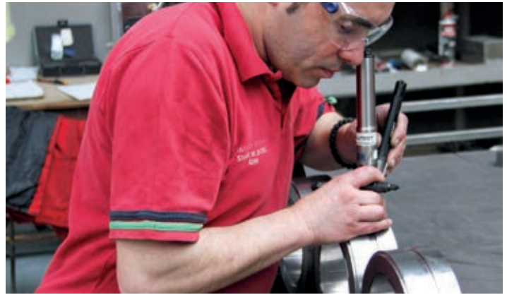
Hardness inspection being conducted on seat ring
