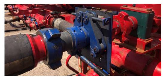
The clamp quick-connect system connected to the frac missile. Using the clamp quick-connect system instead of traditional hammer unions for high-pressure frac hose connections slashed the average makeup time to 20 s, reducing connection time by up to 80%.
