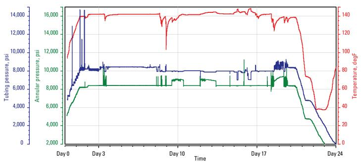
Pressure and temperature measurements obtained by CQG gauges at sensor depth of more than 16,000 ft [4,877 m]. All components of the Quartet system test string reliably performed under high pressure for 20 days.
