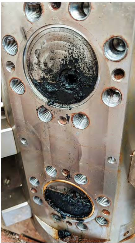
Fig. 2. Body of the venturi section of the surface multiphase flowmeter, where the accumulation of scale and wax can be seen on the membrane of the differential pressure cell. The injection of selected chemicals avoids full plugging of the port and poor transmission of pressure.
