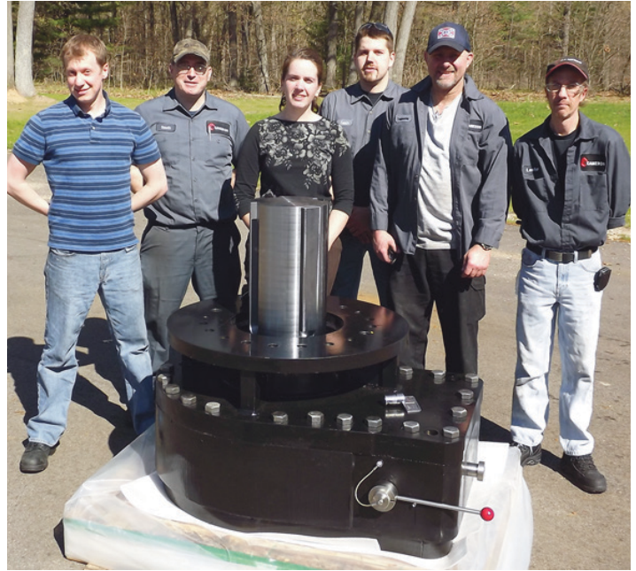
DYNATORQUE D-Stop devices are built for both large and small valves. This DYNATORQUE DT4000 D-Stop device will fit between a large pneumatic actuator and a 36-in, 600-lbm ball valve installed on an offshore platform.
