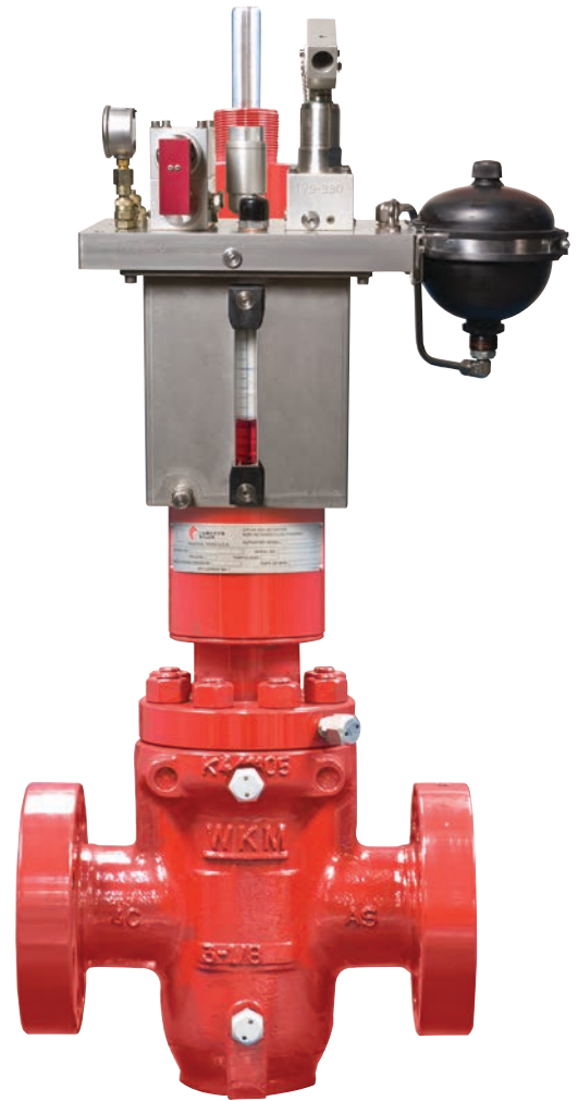
LEDEEN SCCS system mounted on a pedestal for installations in which off-mounting control from actuator provides operational convenience. Requires customer tubing connections to be made between control and actuator for manual or remote trip and between control and pipeline for pilot trip.
