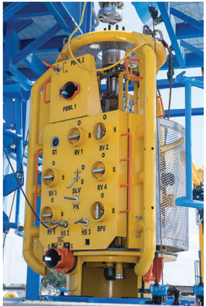
Fluid injection skid
